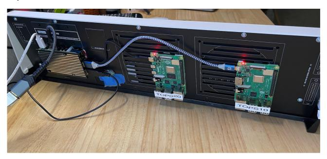
Two less power-hungry Pi 3's (although he used a Pi 4 and a Pi 3) are running headless TOPS-10 and TOPS-20. Of course, they will not drive the front panel, that is reserved for the Pi 5 mounted in the regular way. But the two extra Pi's get their power off the USB ports of the Pi 5, and to connect to the two 'peripheral Pis', Terry uses:
