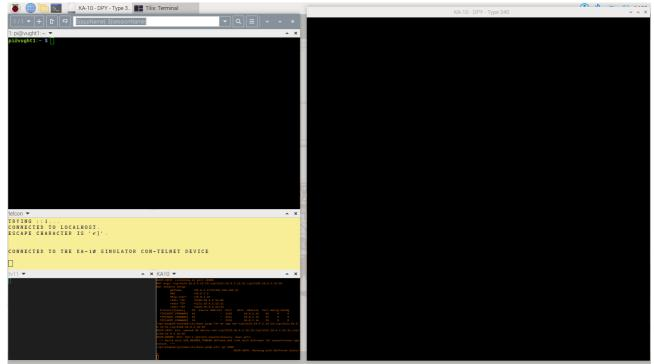
The yellow terminal is the simulated Teletype on the PDP-10's console port. We moved the type340 graphics display to the right. The PDP-10 is running on air at the moment, and to bring up the system: press the **STOP** switch, and then the **READ IN** switch. The latter triggers a PDP-10 to read DSKDMP from paper tape and starts running it.
